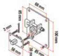
85x100 plate support kit with release and square pin 10 mm
